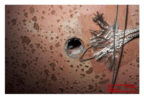
Figure 8. Nose Vent Hole with Thermo Couple After Fast Cook-off
