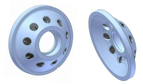
Figure 2. Aft Closure Plate with Polyethylene Plugs
