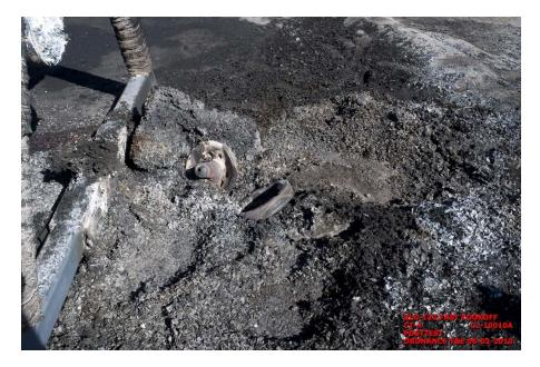
Figure 7. Aft Closure Plate and Retaining Ring Among Ash After Fast Cook-off
