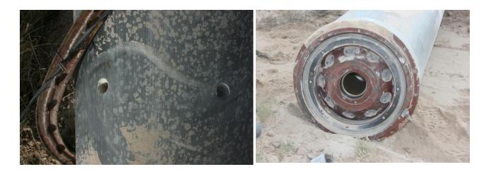
Figure 10. Nose Vent Plugs and Aft Closure Plate Post Sled Test Condition
