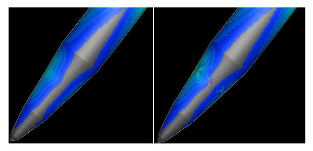
Figure 6. Modeling of No Nose Vents Versus <sup>3</sup>/<sub>4</sub> inch Vent Holes
