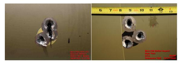
Figure 3. BLU-109 Bullet Impact Test Results
