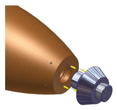
Figure 4. Single Releasing Nose Plug Concept BLU-109
