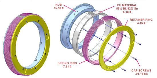
Figure 1. Eutectic Retaining Ring (Exploded View)
